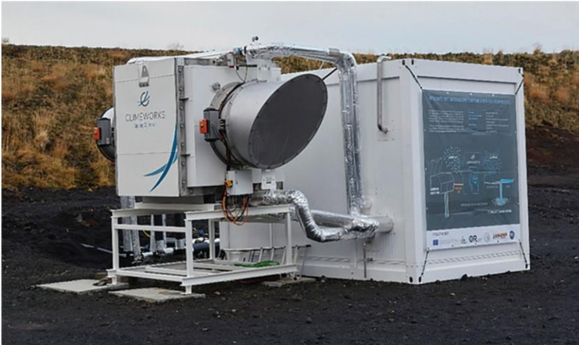
**Figure 4.41** The pilot Direct Air Capture (DAC) unit at Hellisheiði was launched in October 2017. This single unit had the capacity to capture 50 t CO<sub>2</sub> yr<sup>-1</sup>.
